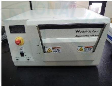
**Fig. 21** Rapid thermal processing system
