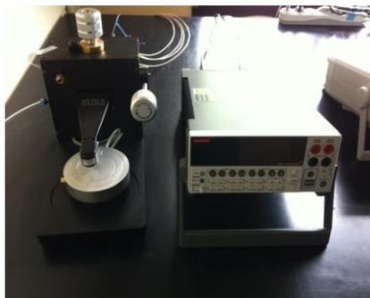
**Fig. 26** Four point probe and sourcemeter using for measuring the resistivity
