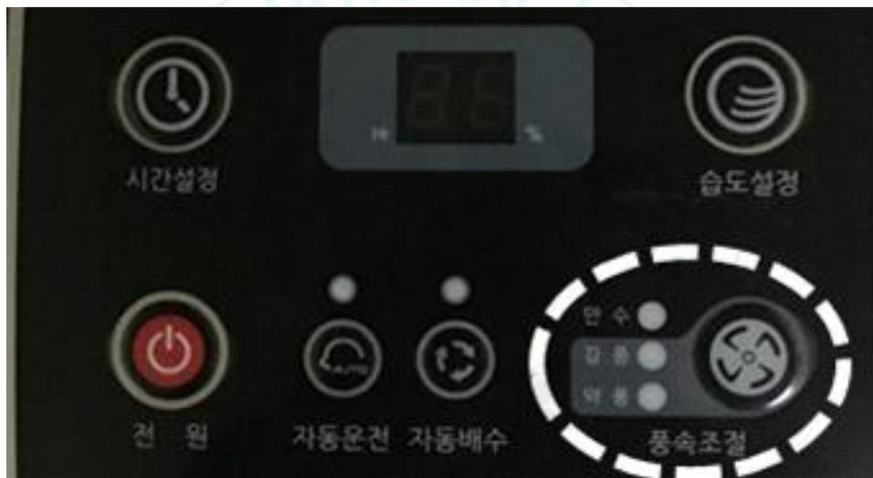
Fig. 7 Wind velocity control button
