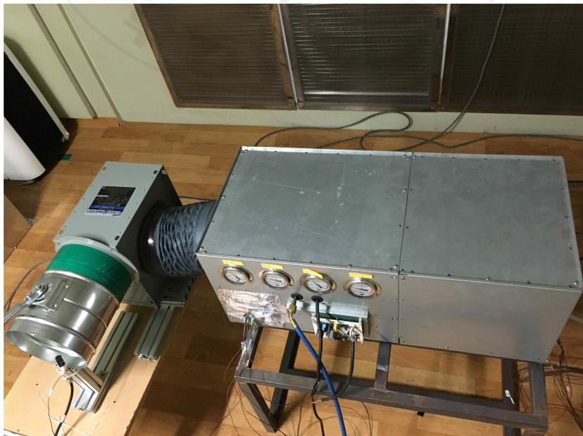
Fig. 8 Sight of refrigeration dehumidifier
