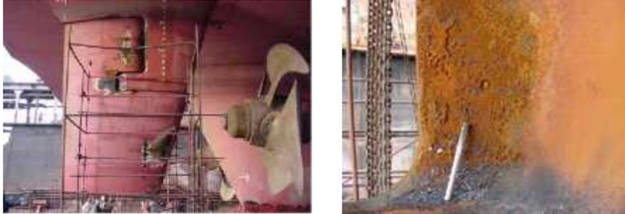
Fig. 1.3. The photographs of cavitation erosion for propeller and rudder of ship.
