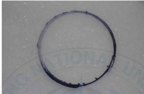
Fig. 2.14 Surface condition of UP coating after 185 min of cavitation erosion test.
