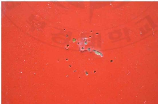
Fig. 2.13 Surface condition of SP coating after 185 min. of cavitation erosion test.
