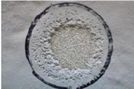
Fig. 2.12 Surface condition of EGP coating after 15 min. of cavitation erosion test.
