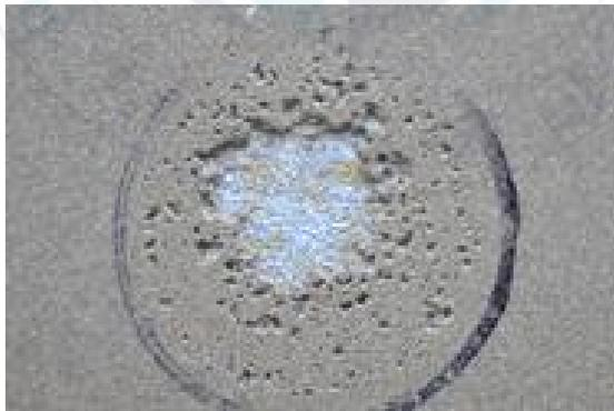
Fig. 2.11 Surface condition of EP coating after 15 min. of cavitation erosion test.
