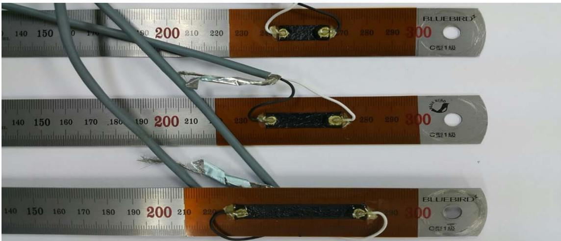
Fig. IV-3 Installation of CNCS (50mm, 30mm, 20mm).
