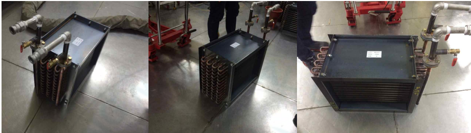
Figure 3.4 Fin-tube radiator manufactured according to the drawings.
