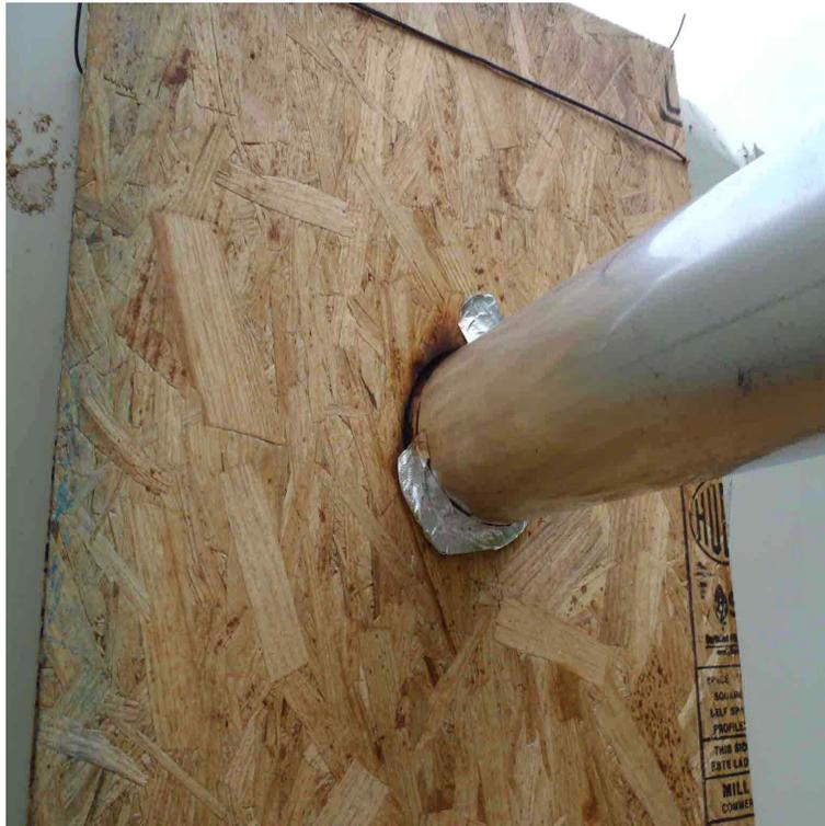
Photo 11 Figure of plywood appears soot after 50 minute.
