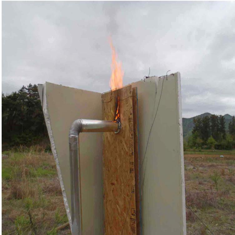
Photo 12 Figure of plywood changed to fire by flare after 123 minutes.
