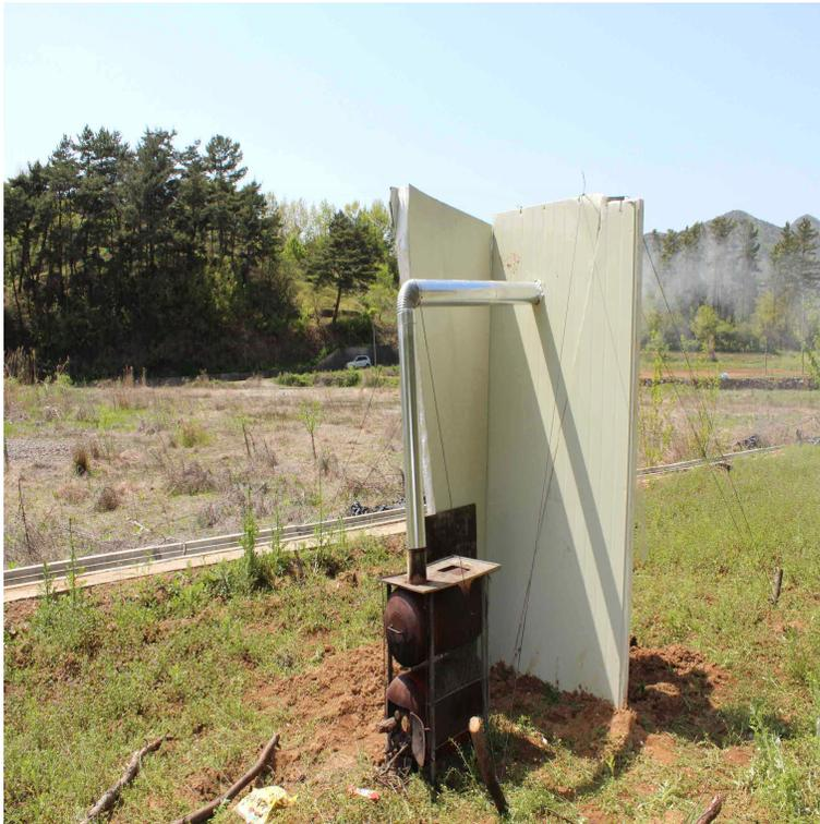
Photo 8 Fire test model of the wood boiler.
