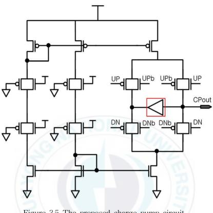
Figure 3.5 The proposed charge pump circuit.
