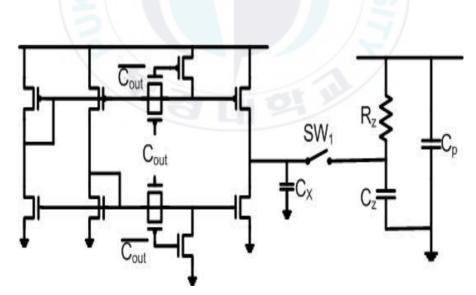
Figure 3.9 The auxiliary charge pump structure.
