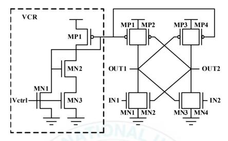
Figure 3.6 The differential delay cell of VCO and VCR.
