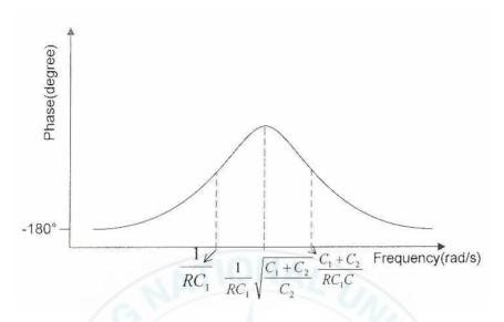
Figure 2.9 The phase characteristics of the third-order PLL.
