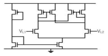
Figure 3.11 The comparator circuit.
