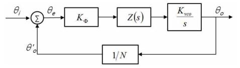
Figure 2.2 The linear PLL model in the locked state.
