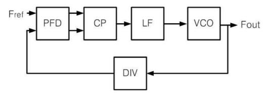
Figure 2.1 Block diagram of the basic phase locked loop.
