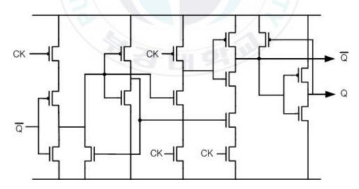
Figure 3.8 The dynamic E-TSPC (Expanded True Single Phase Clock)
