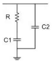
Figure 2.8 The second-order low pass filter.
