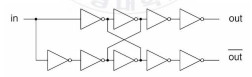
Figure 3.4 The latch buffer circuit.
