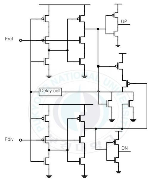
Figure 3.3 The circuit of the PFD.
