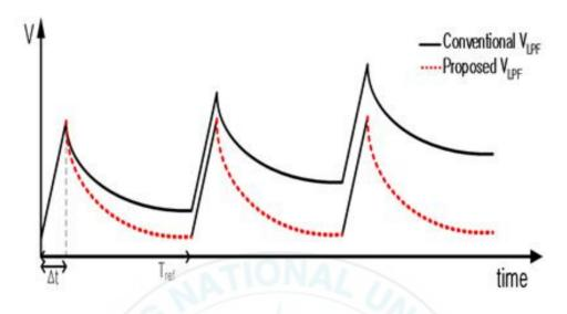
Figure 3.5  $\triangle \triangle V_{LPF}$  of conventional PLL and  $\triangle \triangle V_{LPF}$  of proposed PLL when output voltage of loop filter increases.
