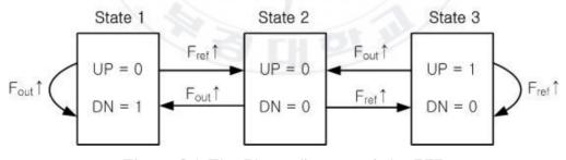
Figure 2.4 The Phase diagram of the PFD
