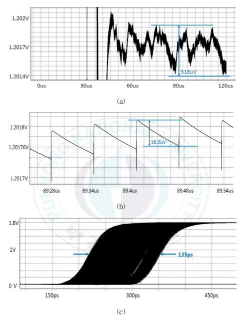
Figure 4.1 Simulation of the conventional PLL's (a)  $\triangle V_{LPF}$ , (b)  $\triangle \triangle V_{LPF}$ , and (c)jitter.
