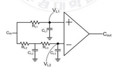
Figure 3.2 The RC time constant circuit.
