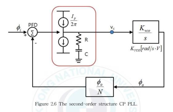
Figure 2.6 shows the basic PLL that has the first-order transfer function on the LPF and VCO. By calculating according to the function in (2–7), the outcome turns out to be what is shown in (2–9).
