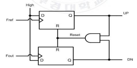
Figure 2.3 Basic structure of the PFD
