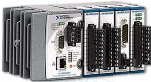
Fig. 4.11 Photo of real-time controller NI cRIO-9024 and modules
