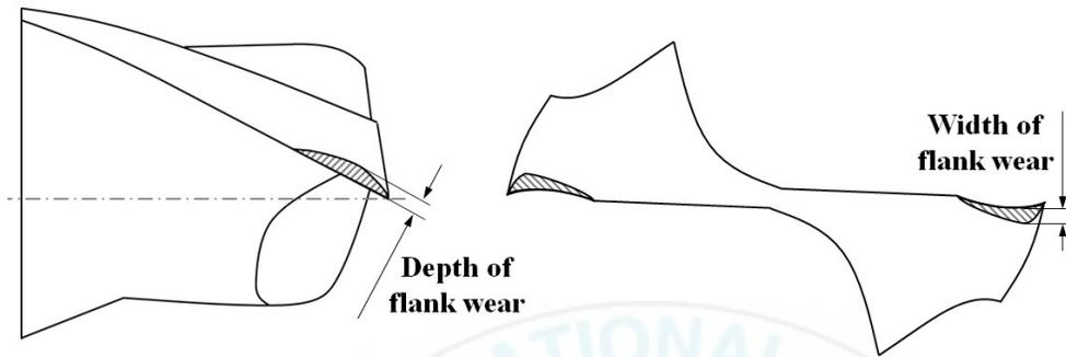
Fig. 3.3 Definition of flank wear on micro end mill
