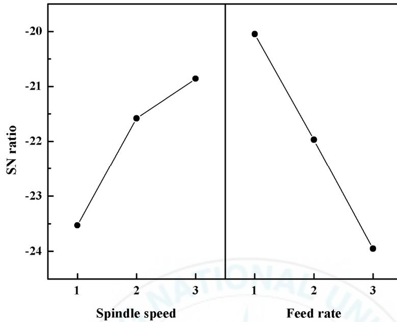
Fig. 4.4 SN ratio on wear of micro end mill
