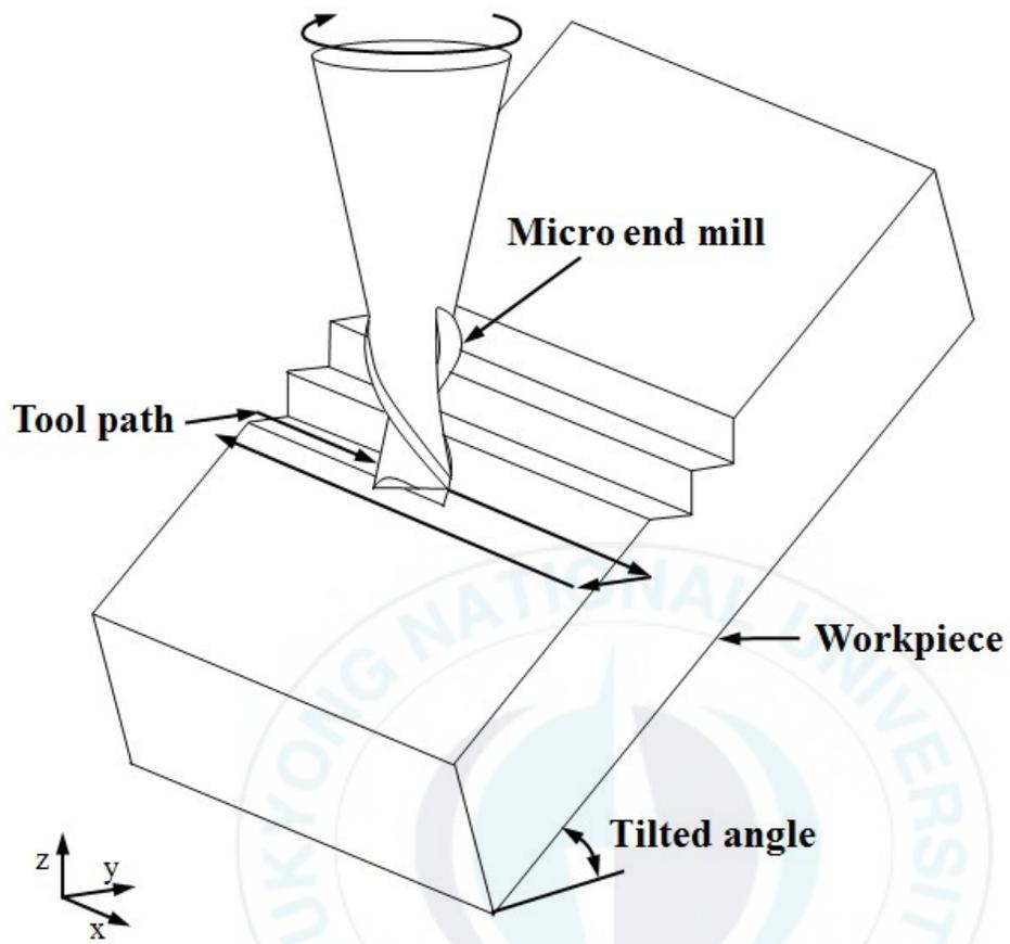
Fig. 3.2 Basic concept of micro prismatic end-milling
