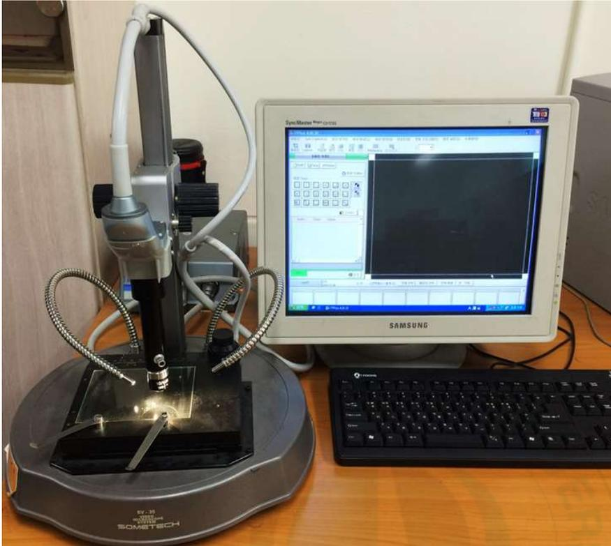
Photo. 3.3 Apparatus of video microscope system
