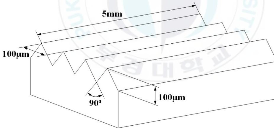
Fig. 3.1 Dimensions of micro prism pattern
