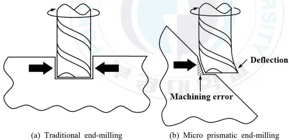
Fig. 4.9 Comparison of cutting force in traditional end-milling and micro prismatic end-milling
