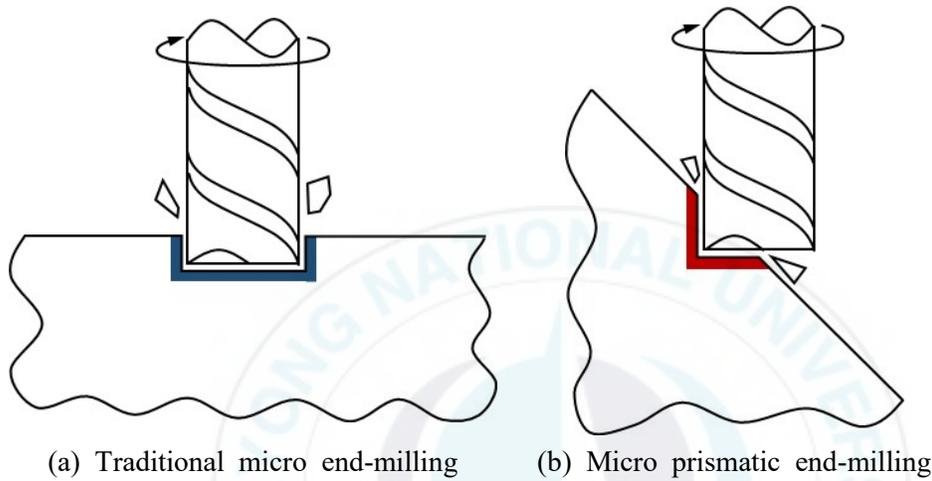
Fig. 2.1 Comparison of traditional end-milling system and micro prismatic end-milling system
