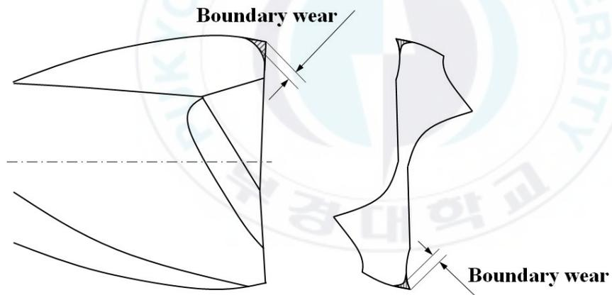
Fig. 3.4 Definition of boundary wear on micro end mill
