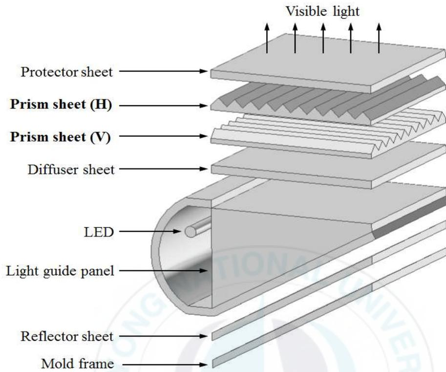
Fig. 1.1 Schematic diagram of back light unit
