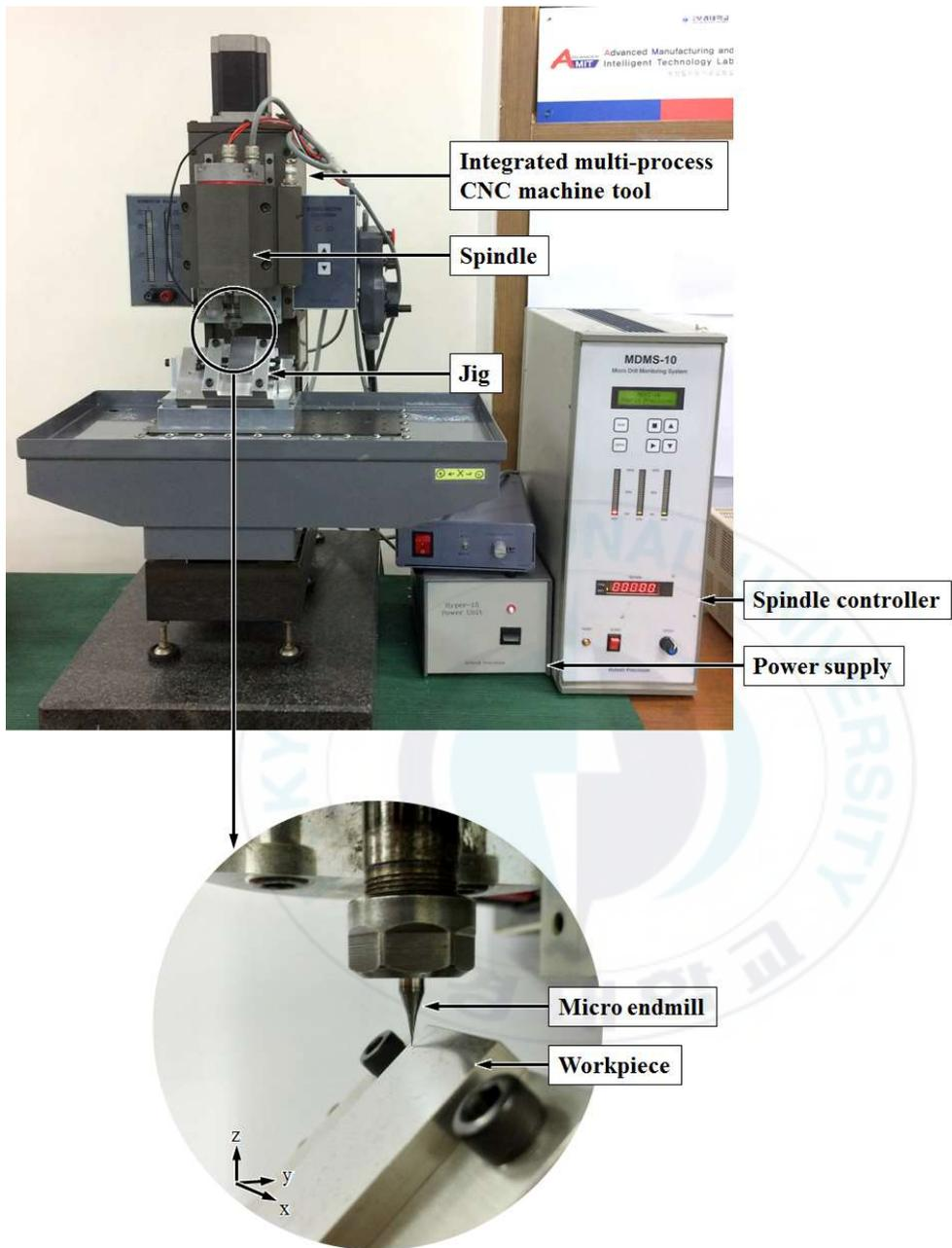
Photo. 3.1 Apparatus of micro prismatic end-milling system
