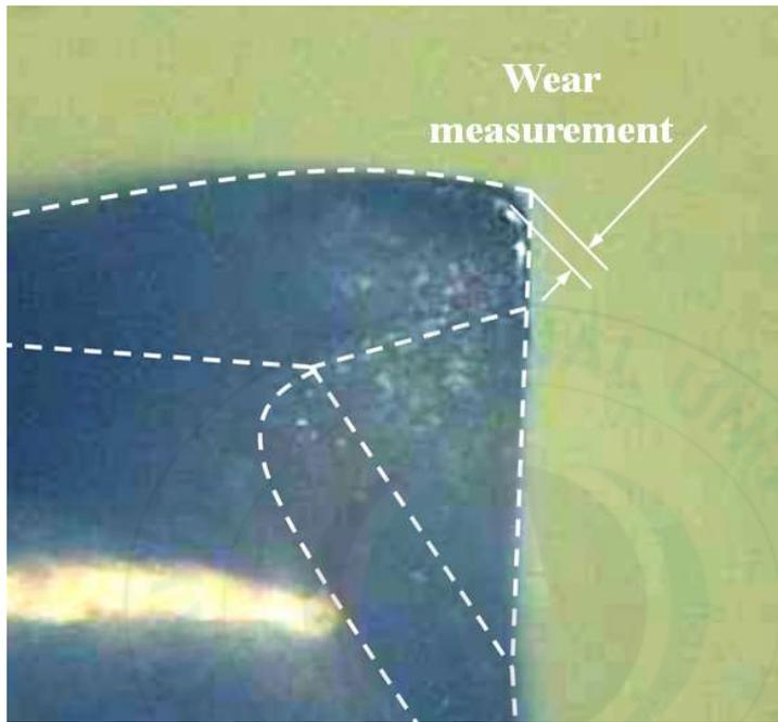
Fig. 3.5 Example of wear measurement
