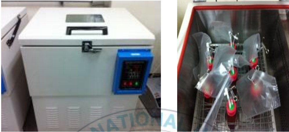
Fig. 4. Photograph of shaking incubator and anaerobic reactor.
