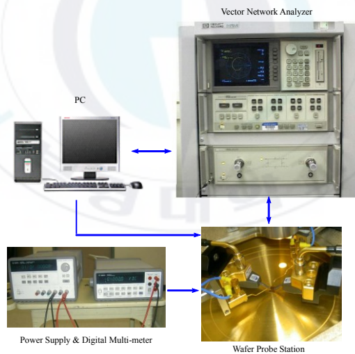
Figure 2.11: S-parameters measurement set-up
