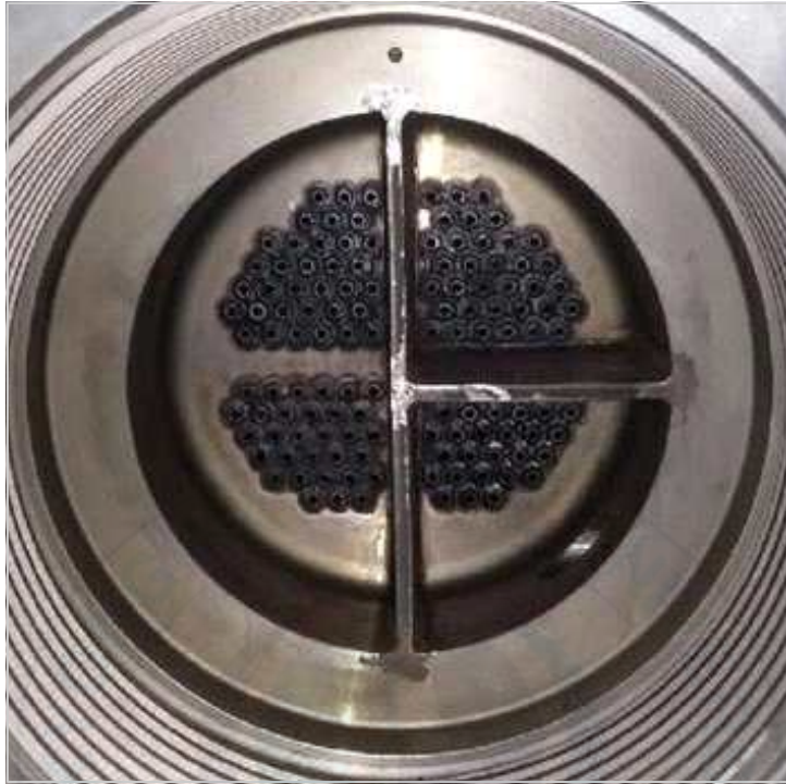
Fig. 2-2 Structure of header and tube arrangement
