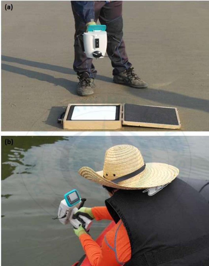
Figure 7. Field spectral reflectance measurement using spectroradiometer : (a) Reference reflectance measurement using spectralon panel and (b) Water(fresh and algal bloom) reflectance measurement.
