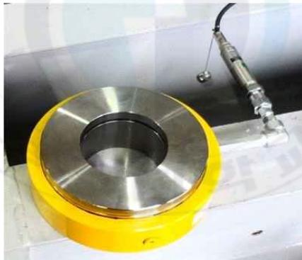
(c) Pressure-type loadcell
