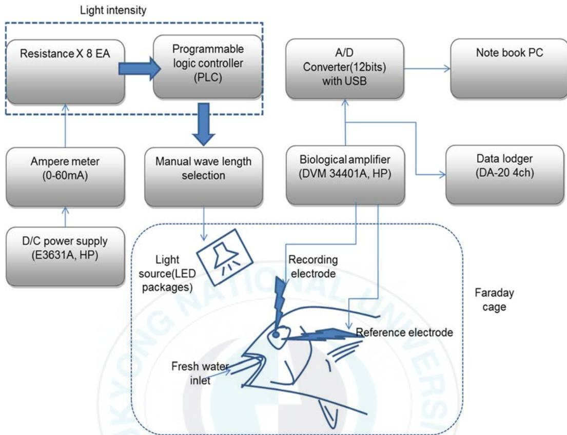
Figure 4. Schematic representation of equipment setup for ERG recording.
