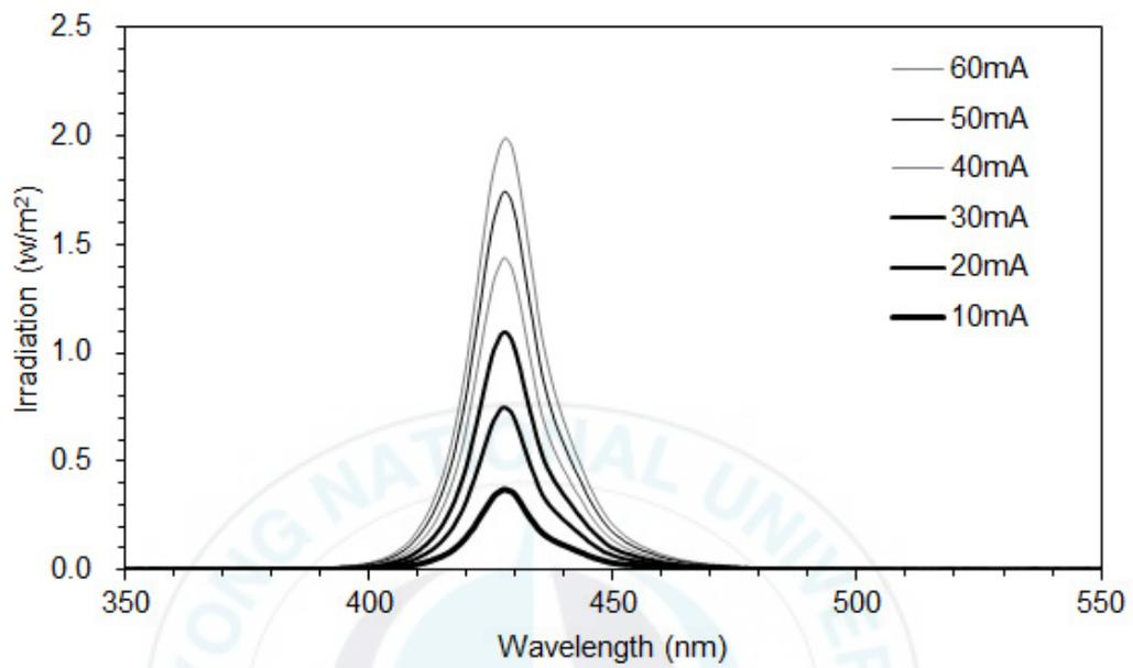
Figure 5. Measured relative spectral power curves from 428 nm LED package.
