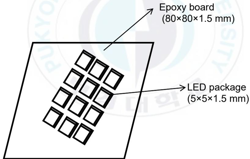
Figure 2. Arrangement of LED packages attached on an epoxy board.
