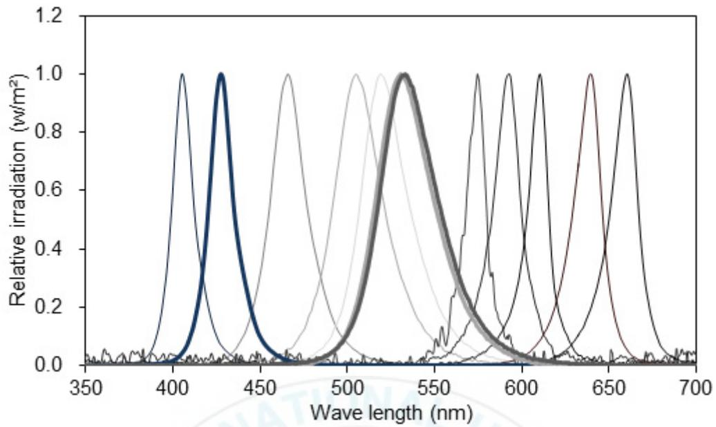
Figure 1. Measured relative spectral sensitivity curves of LEDs used in the experiment.
