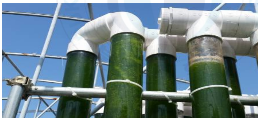
Figure 2. Photo images of the vertical photobioreactor system used in this study showing Chlorella vulgaris cultivation.
