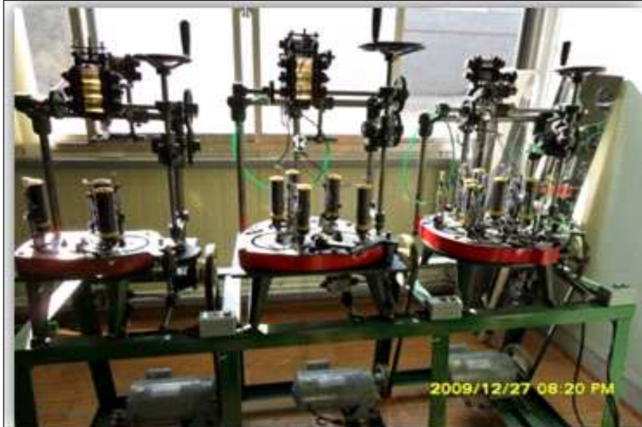
(a) Knitting machine of carbon fiber bundle
