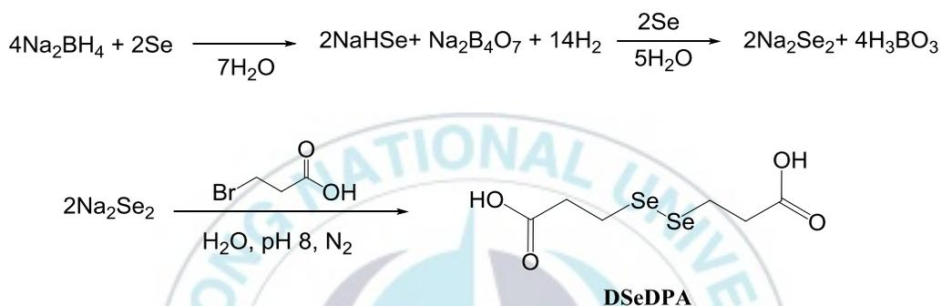
**Scheme 2.1** Synthetic route for 3,3'-diselanediyldipropionic acid proposed by Cheng<sup>9</sup>
