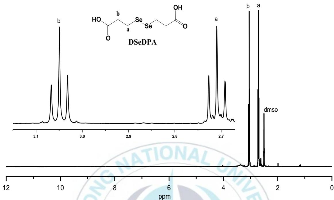
**Figure 2.1** <sup>1</sup>H-NMR spectrum of 3,3'-diselanyldipropionic acid
