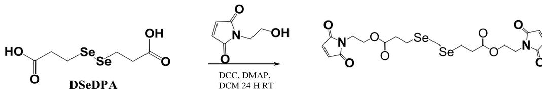
**Scheme 2.3** Synthetic route for diselenide bismaleimide containing crosslinker( Bis(2-(2,5-dioxo-2,5-dihydro-1H-pyrrol-1-yl)ethyl)3,3'-diselanyldipropionate)
