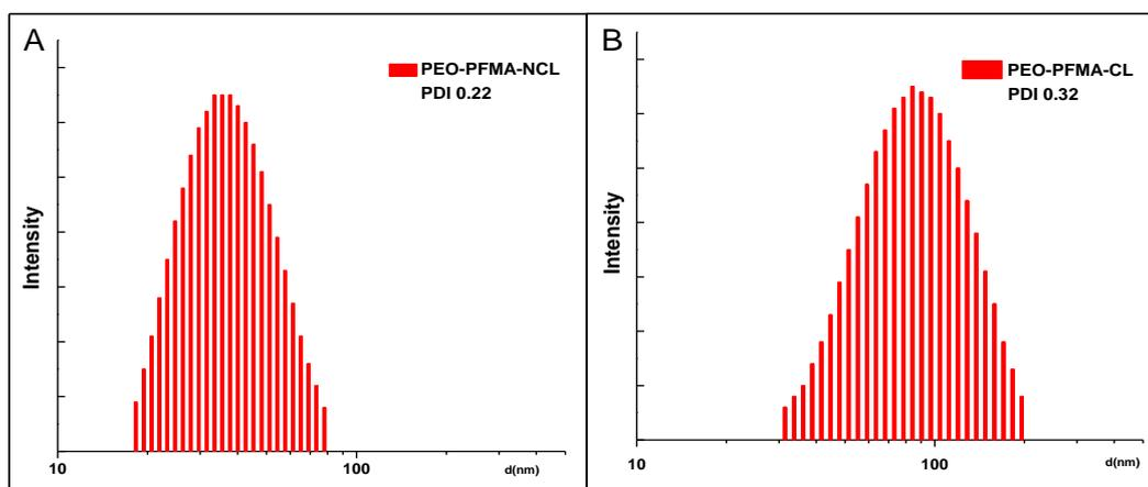
**Figure 3.4** DLS spectra of (A) non-core-crosslinked micelles, (B) core-crosslinked micelles
