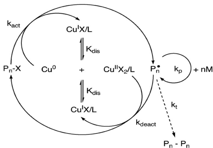
**Scheme 1.1** The SET-LRP mechanism as proposed by Percec et al.<sup>9</sup>.
