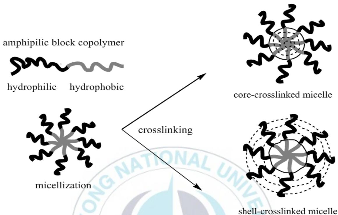
**Figure 1.2** Representation of formation of shell-crosslinked or core-crosslinked micelles
