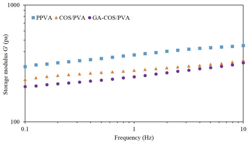
Fig. 12. The graph of the storage modulus vs frequency of PPVA, COS/PVA and GA-COS/PVA
