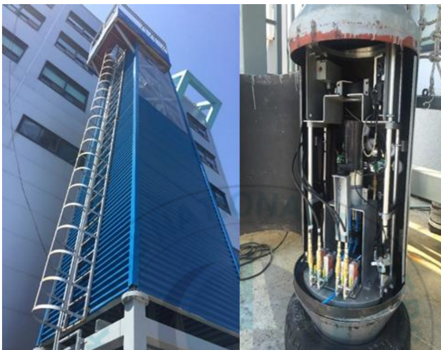
Fig. 2 (left) overall facility of drop tower and (right) experimental setup in drop tower capsule.
