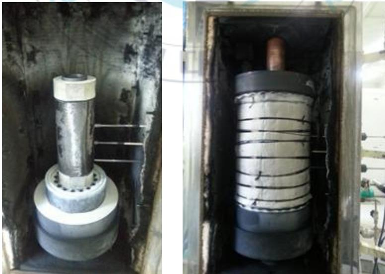
**Fig. 3-3** Photographs of the TG-CVI reactor considered in this study.
