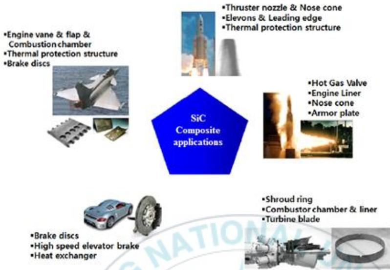
Fig. 2-1 Applications of SiC composite materials.
