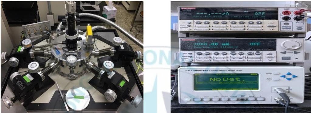
Figure 18. Vacuum probe station in our lab and Kethley Source-Measure Unit
