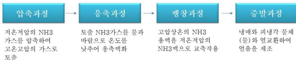
Figure 1. The refrigeration manufacturing process flow
