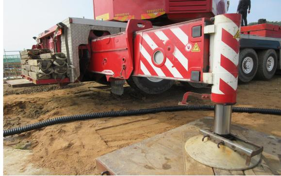
Fig. 2.5 The outrigger of the mobile cranes
