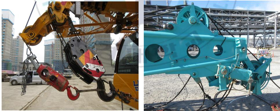
Fig. 2.2 Anti-rotating and overload protection device for mobile cranes
