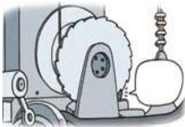
Check the installation status of the traction machine
