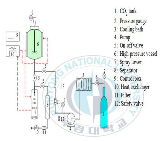
Figure 4.1. Schematic diagram of PGSS process.
