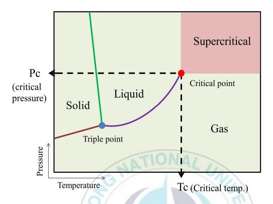
**Figure 1.12**. Pressure-temperature phase diagram of a substance with critical temperature (Tc) and pressure (Pc)
