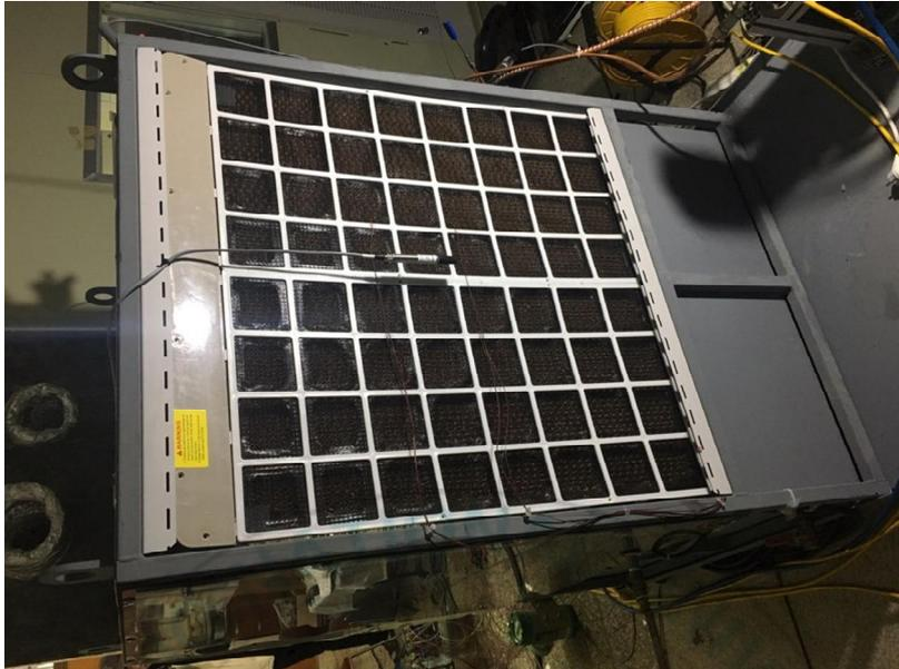
Photo. 2.2 Evaporating part of hybrid cooling system
