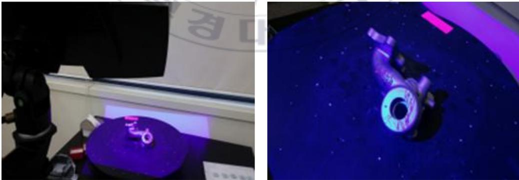
Fig. 5.6 Measuring 3D scan of turbo charger housing
