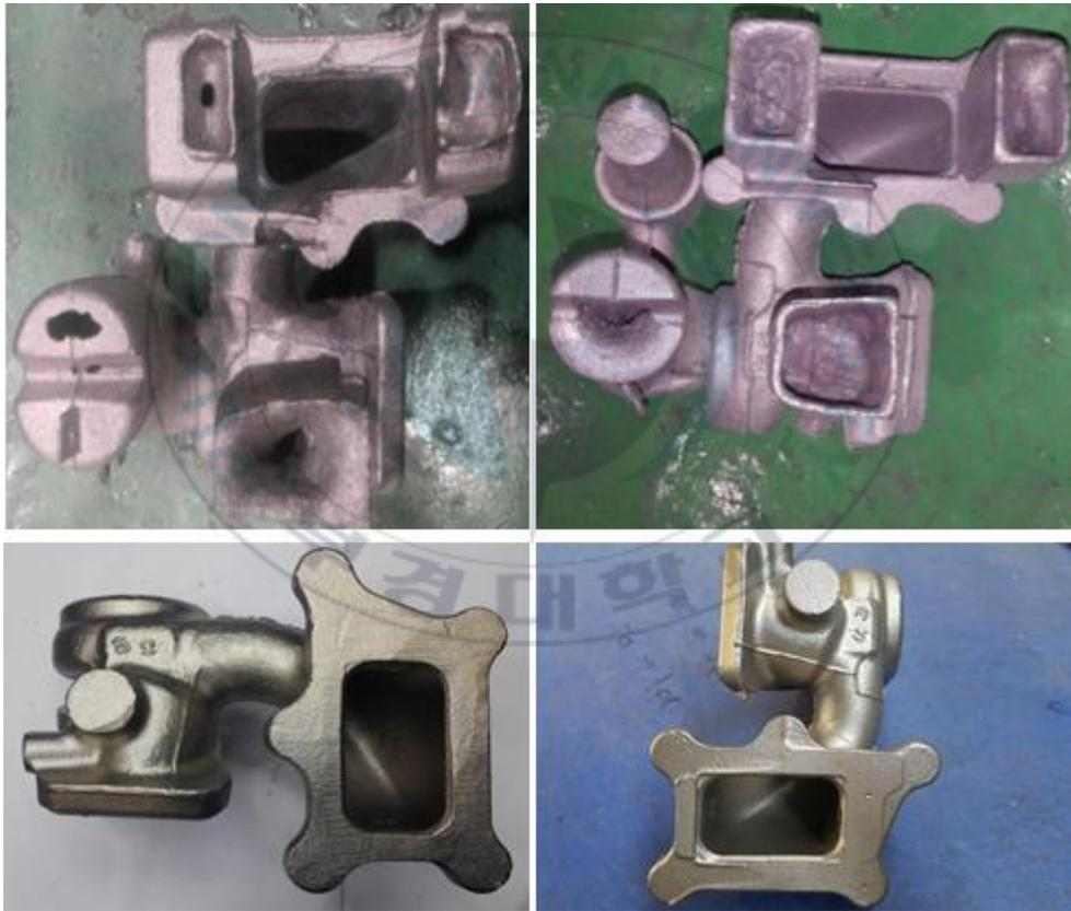
Fig. 5.2 Casting turbo charger housing - case 1
