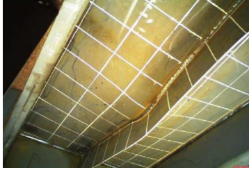
Before fracture: test (Alsos and Amdahl, 2009)
