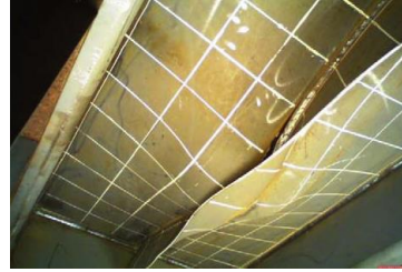
After fracture: test (Alsos and Amdahl, 2009)
