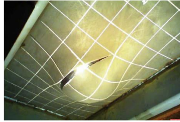
After fracture: test (Alsos and Amdahl, 2009)
