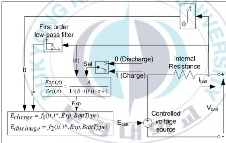
Figure 9 Equivalent circuit of battery with in Matlab Simulink[32], [33]
