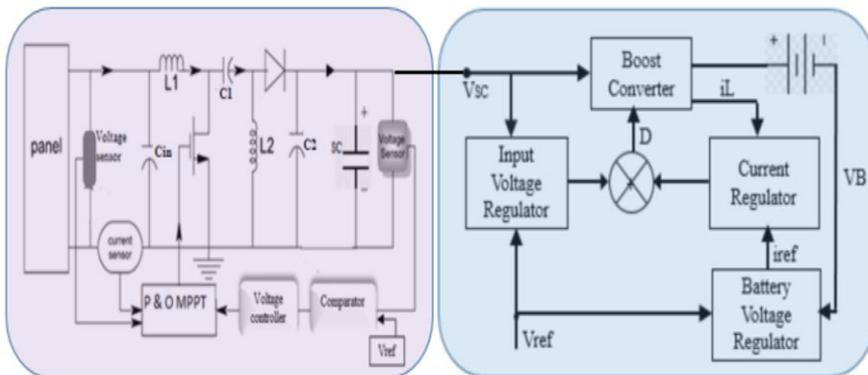
Figure 19 Model of hybrid charging system
