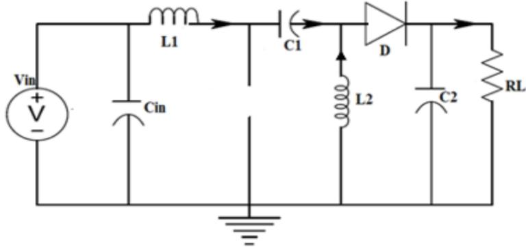
Figure 13 Open mode of SEPIC converter.
