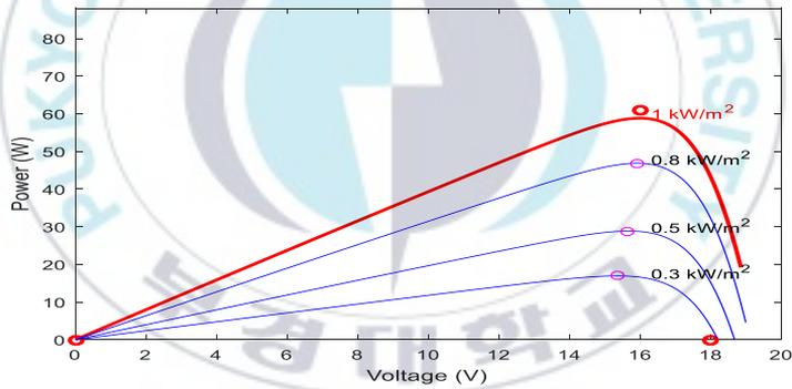
**Figure 26 P-V curve of solar module on variable irradiance**
