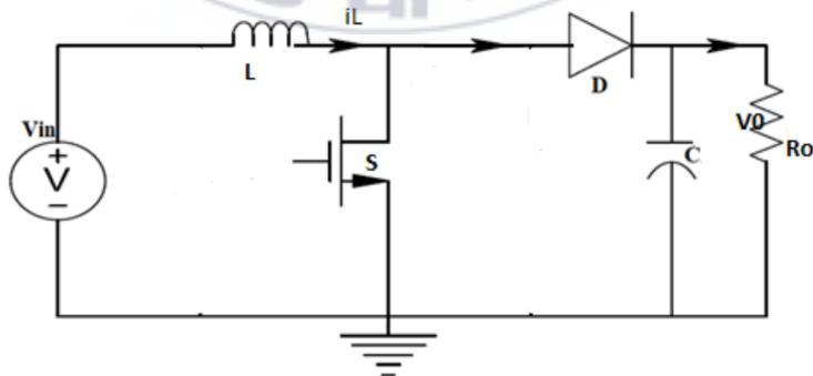
Figure 14 DC-DC Boost Converter Topology
