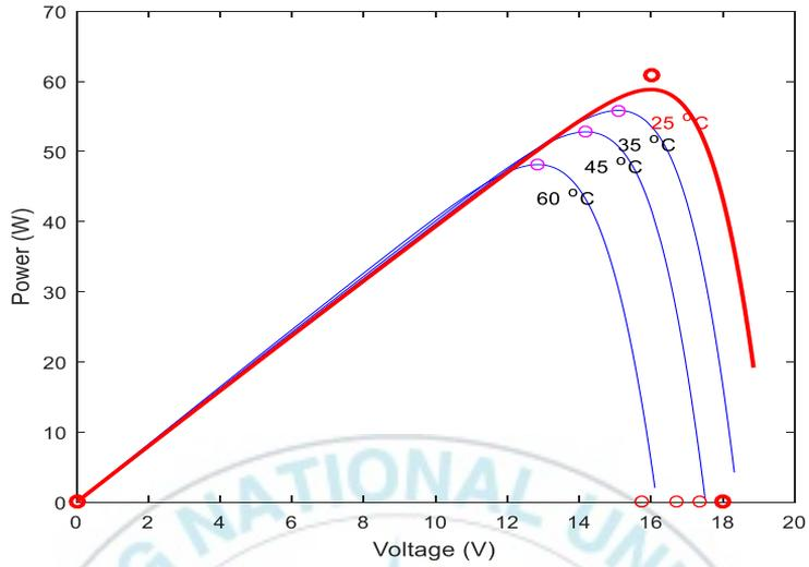
Figure 29 P-V curve of solar module on variable temperature input
