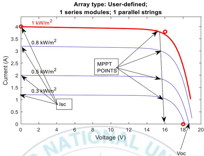
**Figure 25 I-V curve of solar module on variable irradiance**
