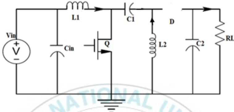
Figure 12 Closed mode of SEPIC converter
