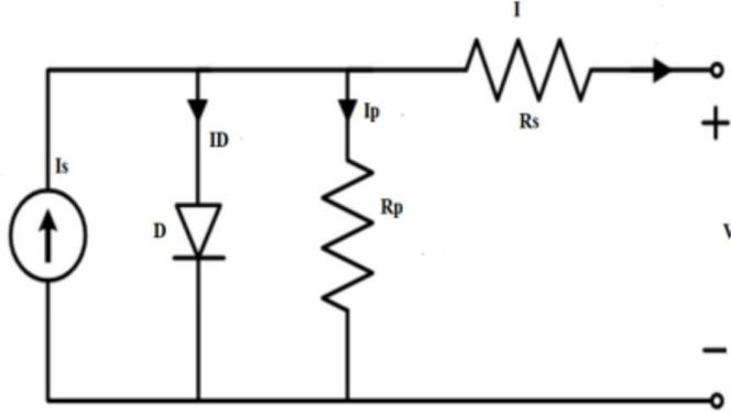
Figure 4 The PV cell equivalent circuit
