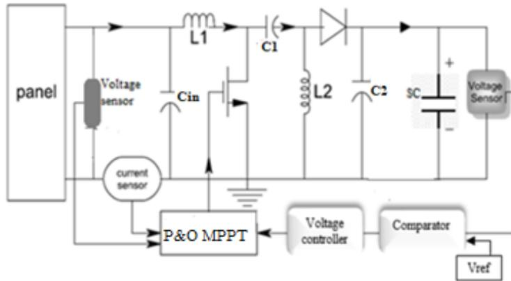
**Figure 17 Model of MPPT Supercapacitor Charging System**
