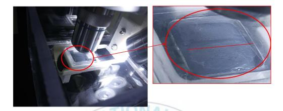
**Fig. 6-11** Movement of the microbubbles under the acoustic pressure by the line-focused source. It can be seen clearly that the microbubbles was separated in both sides of the focused line position.
