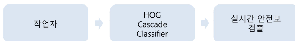
Fig.11 Real-time safety helmet detection using HOG Cascade Classifier
