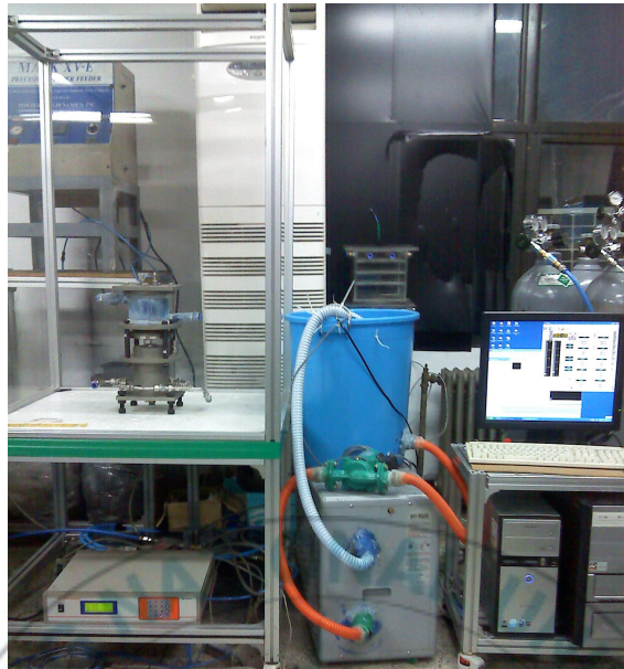
Fig. 3.2 Experimental apparatus of counterflow burner
