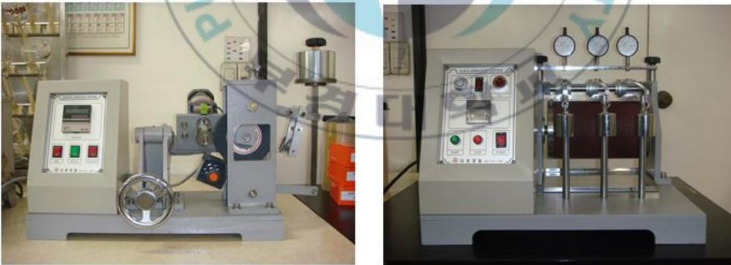
Figure 10. Picture of Akron & NBS abrasion tester.
