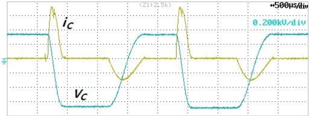
Fig. 4-21 Measured i_c and V_c waveforms of recharging mode
