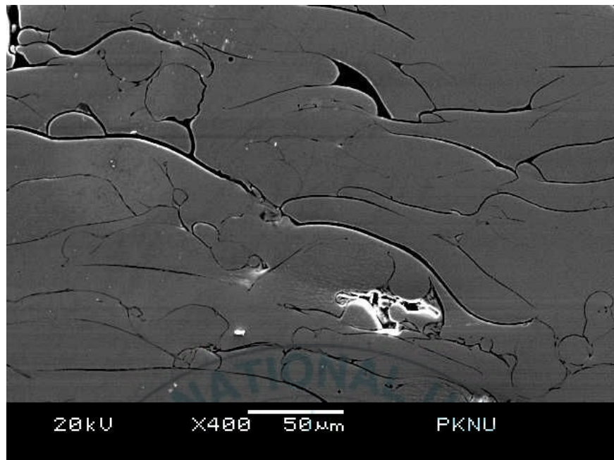
Fig.7 Microstructure of as-sprayed coating layer
