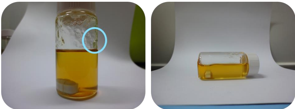
Figure 22. Gelation due to the reaction of KD-1 dispersant with EC
