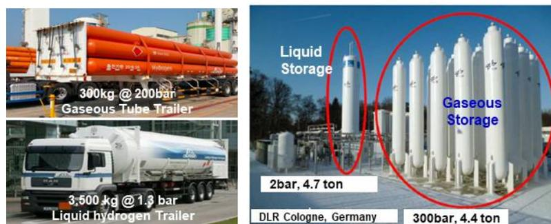
**Fig. 1.10** Comparison of gaseous and liquid hydrogen
