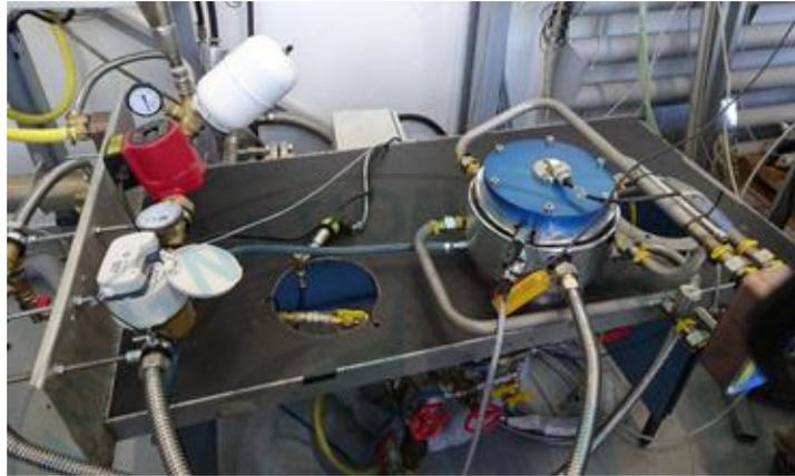
(a) Test equipment for cryogenic turbo expander
