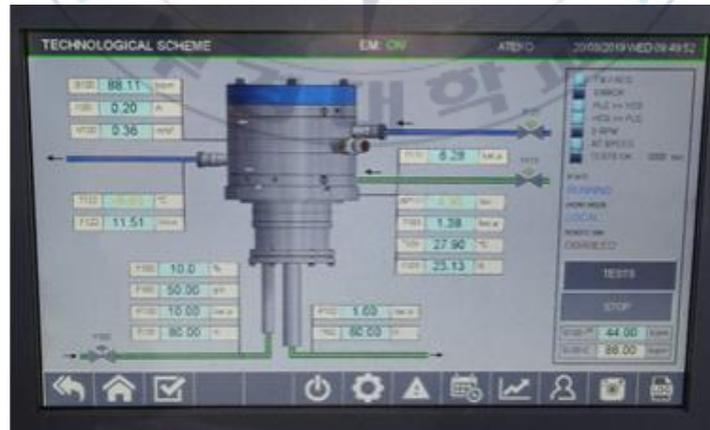
(a) Control system for cryogenic turbo expander
