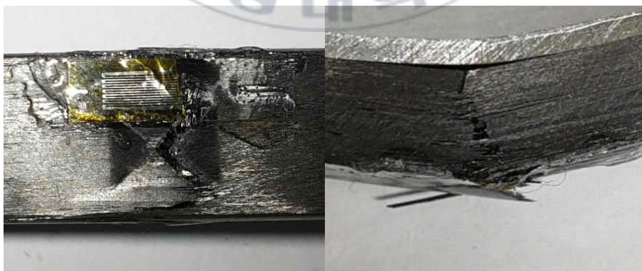
Fig. 15 Fracture shape of T1 specimen
