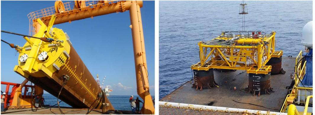
Figure 6-18. Example of the actual subsea installation system (left: suction pile, right: manifold)
