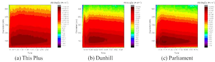
Fig. 4.18 Measurement of nanoparticles in indoor air by SMPS when volunteer 1 smoked conventional cigarettes
