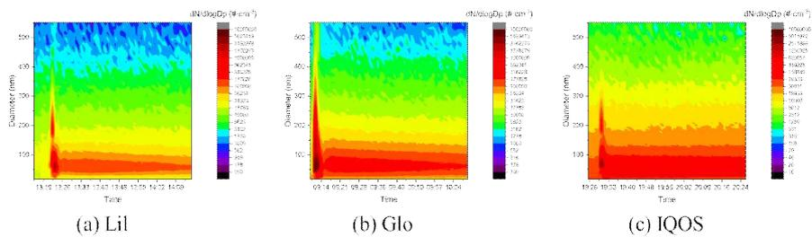
Fig. 4.17 Measurement of nanoparticles in indoor air by SMPS when volunteer 2 vaped heat-not-burn tobacco
