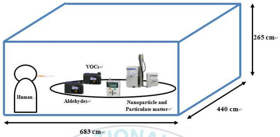
Fig. 3.2 Simulated office chamber system for secondhand smoke experiment
