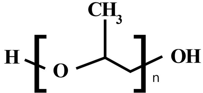
Fig. 2.1 Structural formula of propylene glycol (PG)
