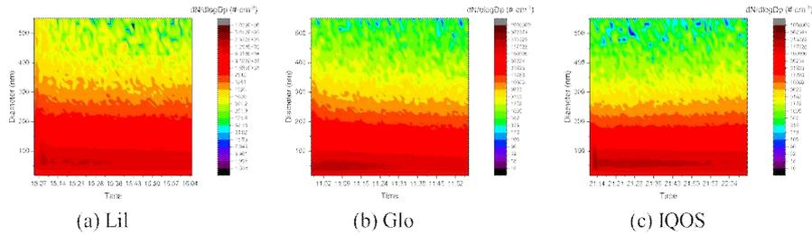
Fig. 4.15 Measurement of nanoparticles in indoor air by SMPS when volunteer 1 vaped heat-not-burn tobacco
