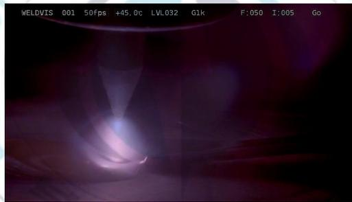
Fig. 4.2 Snap shot of Arc length 6mm, Filler height 0mm
