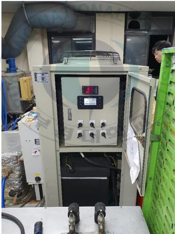
Figure 2 Water side thermostat
