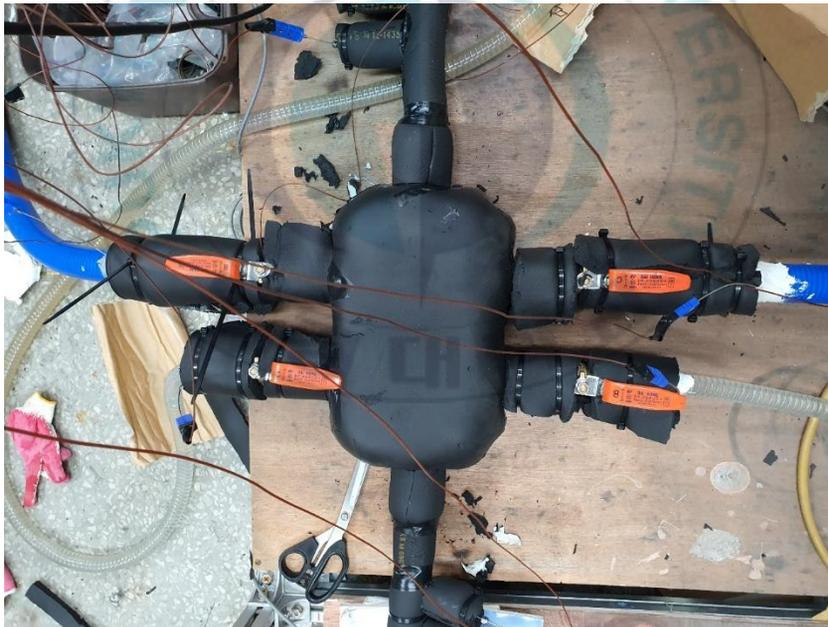
Figure 6 Multi-stream heat exchanger after insulation
