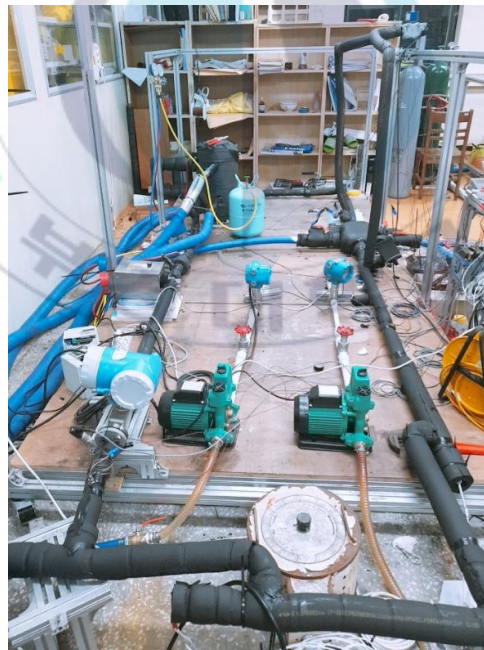
Figure 2 Multi-stream PFHE experimental apparatus
