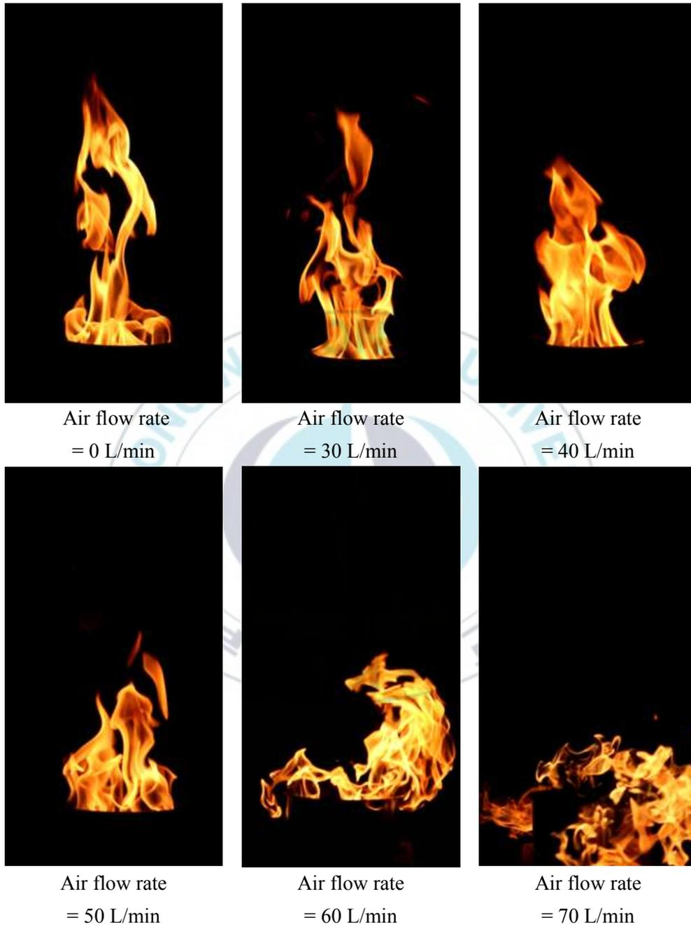
Figure 23. Visualization of heptane pool fire during discharge of air (Fire source diameter = 160 mm).
