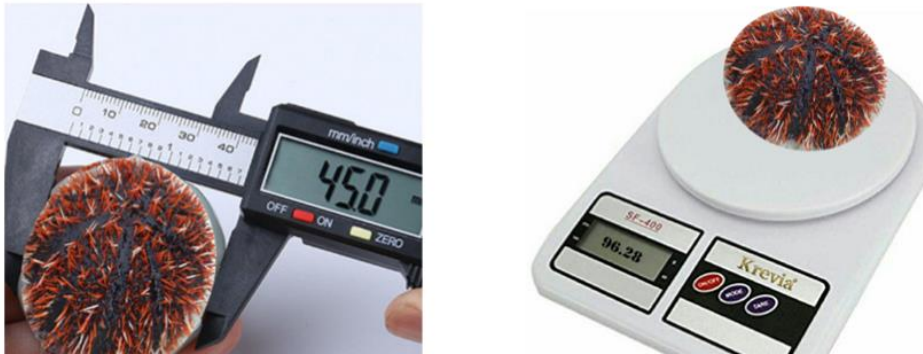
Figure 9. The measurement of T. gratilla using digital electronic vernier caliper on the left and electronic weighing balance on the right
