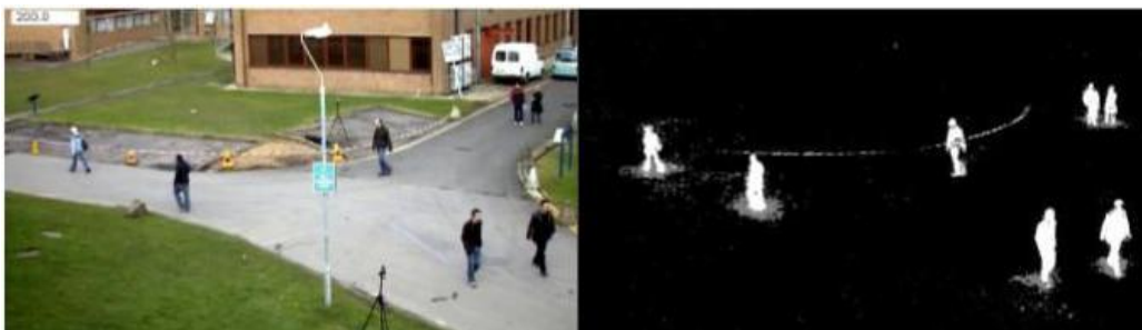
Fig 9. Left: Original Image; Right: Background subtracted binary image using the MOG2 technique
