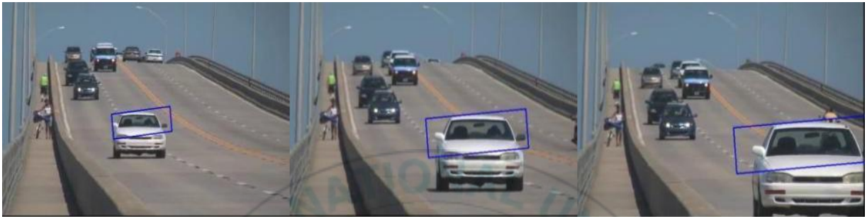
Fig 8. Camshift based object tracking
