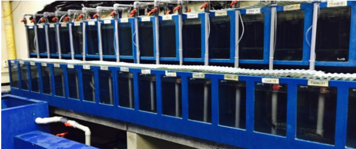
Figure 2-2. The experimental tanks (22×47×32 cm) used for rearing of whiteleg shrimp for eight weeks, fed by the eight experimental diets.
