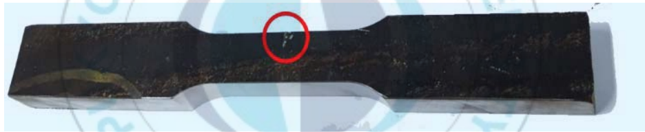
Figure 5 Defect on No.1 specimen
