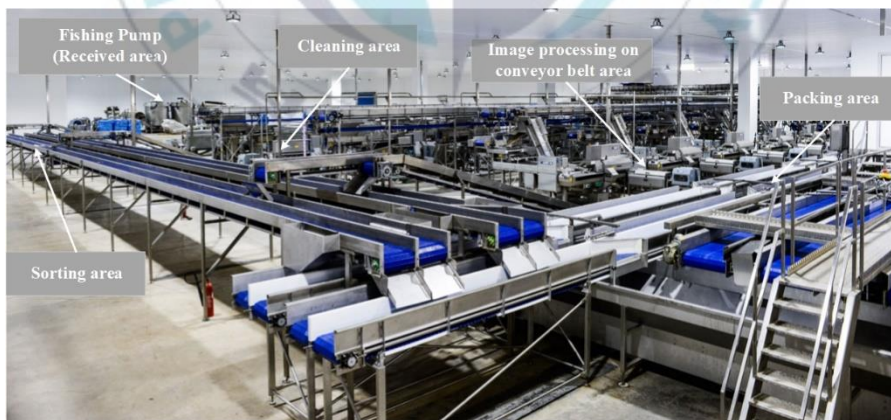
Fig. 2.1 Fish conveyor fish line at Pelagic factory
